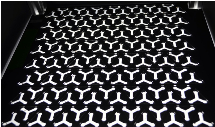
Fig. 6. Y-maze arrays of a high-throughput device for studying the body lateralization of 95 fruit flies simultaneously.
