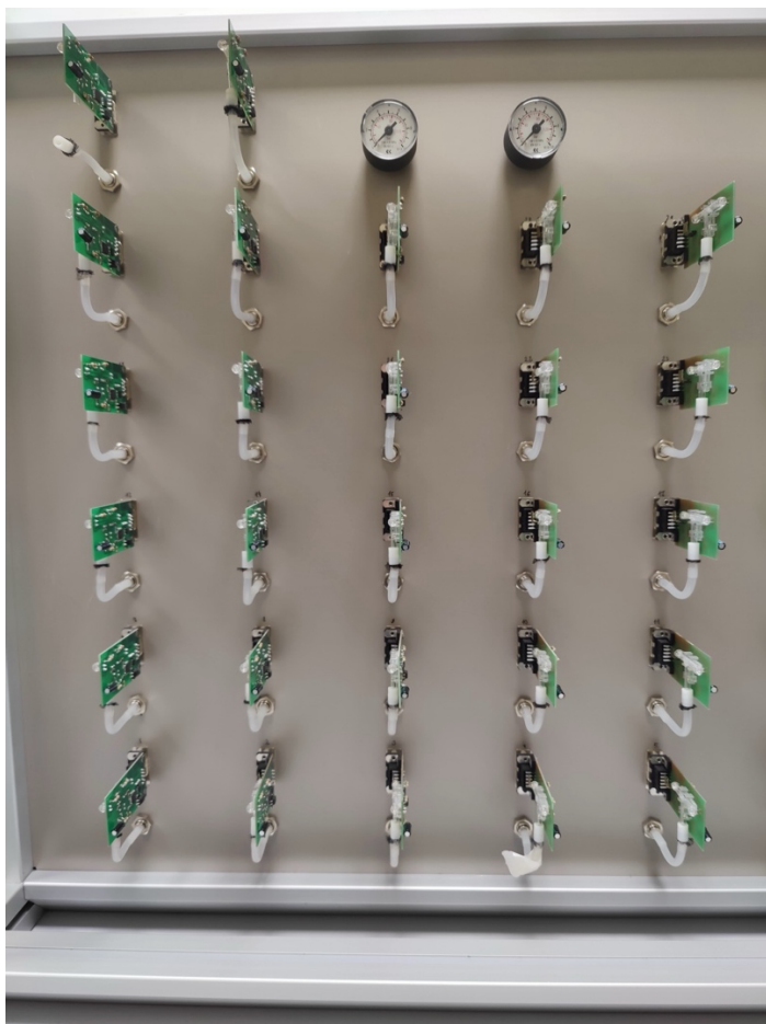
Fig. 2. The 27 individual modules to study phototaxis in 27 fruit flies simultaneously.
