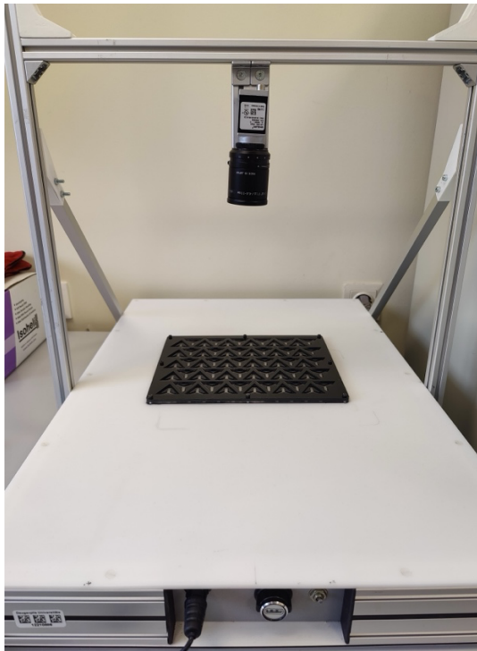
Fig. 9. An array of 60 individual Y-mazes and a video camera is set for a handedness experiment.
